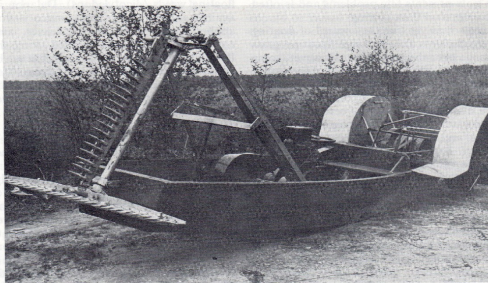
Fig. 364 Mechanical weedcutter with horizontal and vertical beams. It is motor driven and equipped with paddle wheels at the back. Valkenswaard fish farm, the Netherlands.
